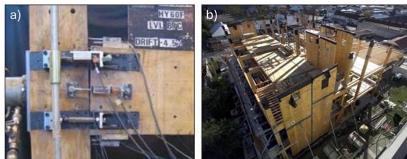
Figure 3. a) Example of experimental test on a beam-column joint based on the Pres-Lam technology [4], and b) NMIT Arts & Media Building realized by implementing the Pres-Lam technology [9].
