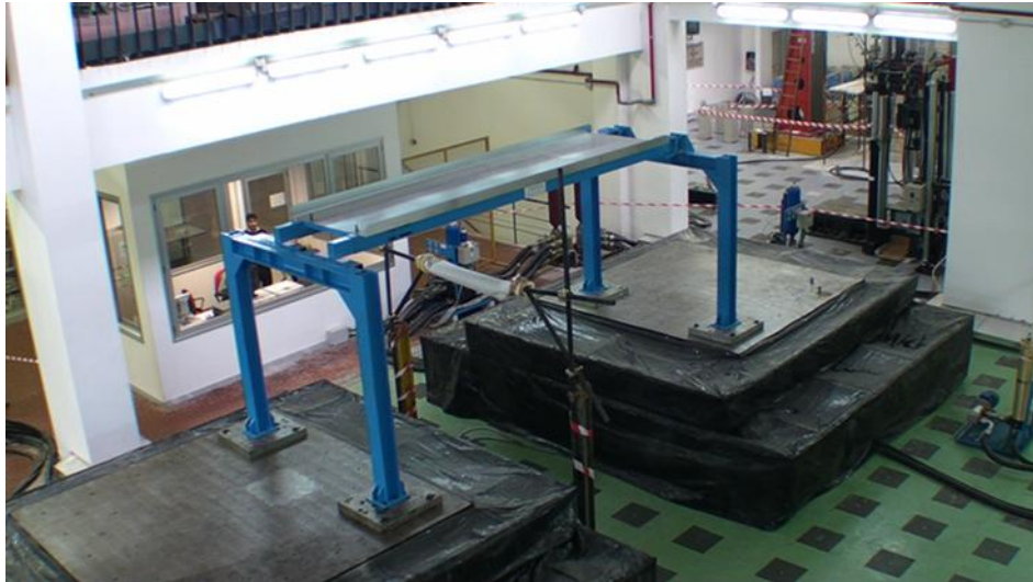
Figure 6. Shaking tables available at DiST laboratory.
