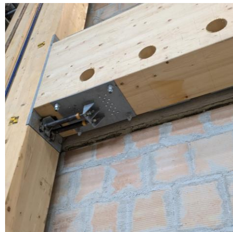
Figure 19. Pres-Lam beam-column connection with a steel-based reinforcement for the timber joint: (a) schematic illustration and (b) example of implementation for experimental tests part of the MULTICARE research project.
