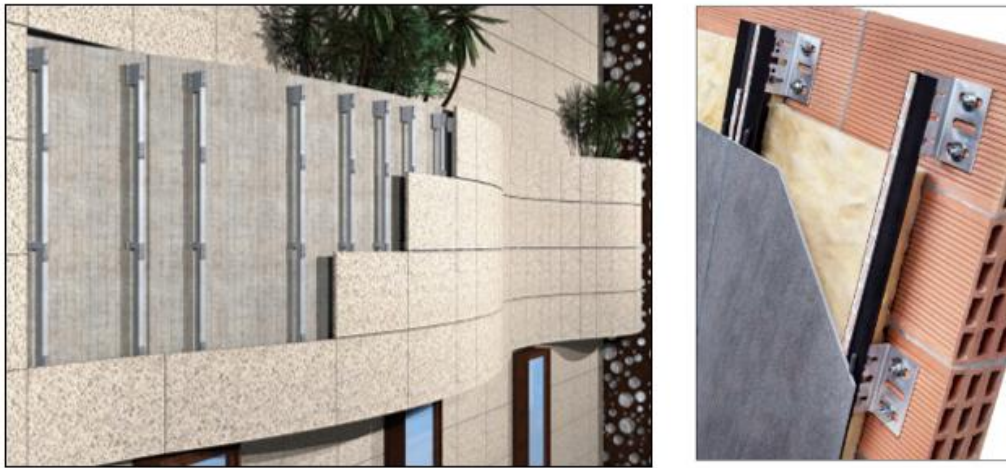
Figure 33. Example of a traditional ventilated facade.
