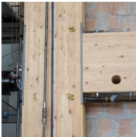
Figure 19. Pres-Lam beam-column connection with a steel-based reinforcement for the timber joint: (a) schematic illustration and (b) example of implementation for experimental tests part of the MULTICARE research project.
