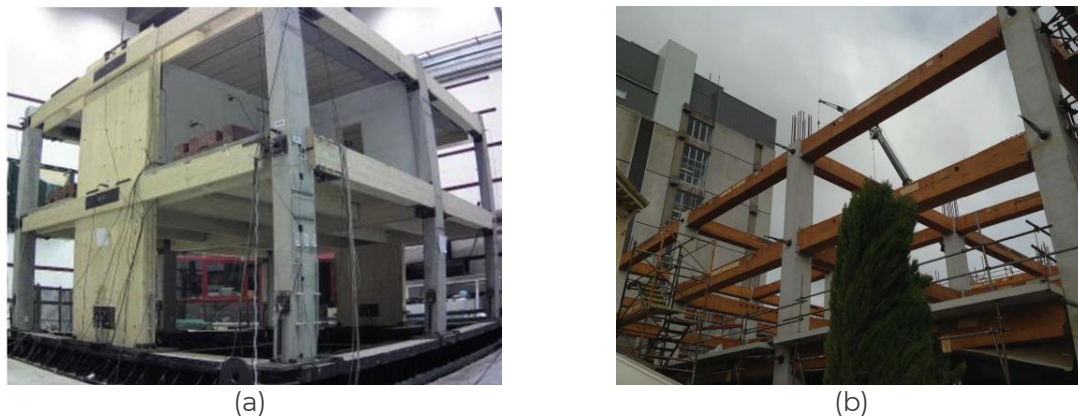
Figure 16. Hybrid concrete-timber post-tensioned solutions: (a) experimental specimen (after Pampanin et al., 2023), and (b) example of implementation for a real building.
