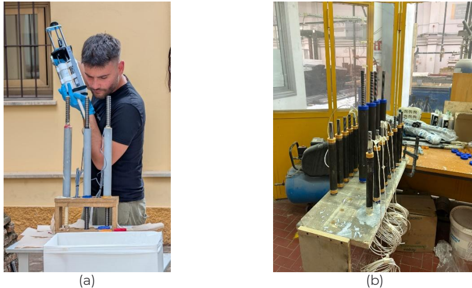
Figure 18. Example of (a) the filling operation for “Plug-and-Play” dissipaters with epoxy, and (b) the assembled devices.
