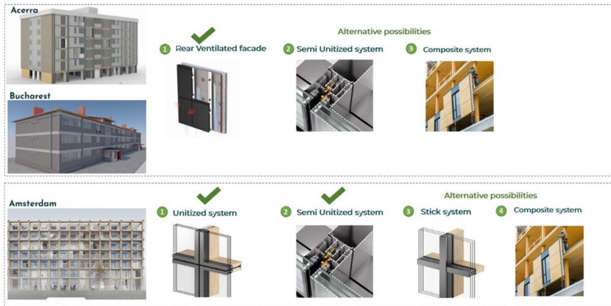
Figure 3 Selected facade systems for demonstrator projects.
